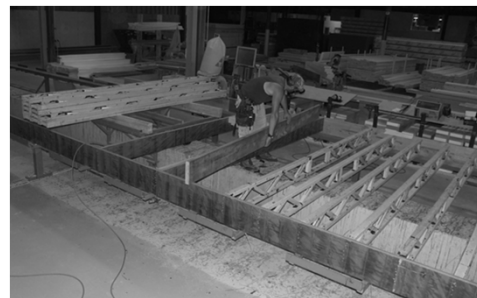
Beginning of floor system-open web joists, LVL to reduce columns in basement
