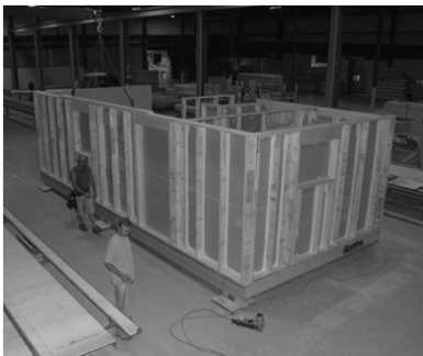
Assembled walls on floor for 1/2 of 1 st floor
